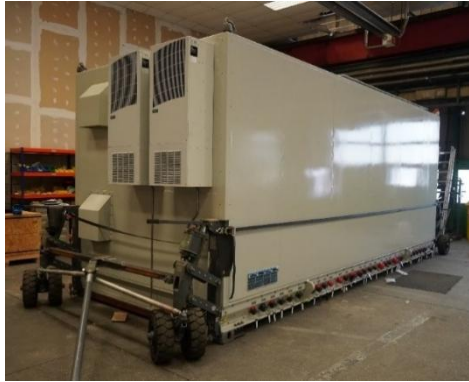
Gas turbine control house VT Systemtechnics
